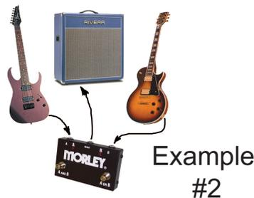
GROUND LOOP NOISE? Hooking two amps together via an ABY box can sometimes create a LOOP ANTENNA which causes hum (also known as Ground Loop Hum, 60Hz Hum or 60 Cycle Hum, 50Hz in Europe). This is not caused by the ABY but by the connection of two amp grounds via the ABY. If this does occur, it can be easily corrected. Visit [www.ebtechaudio.com](http://www.ebtechaudio.com) for information on eliminating Ground Loop Hum & Noise with our Hum X or outside North America, the Hum Eliminator.
