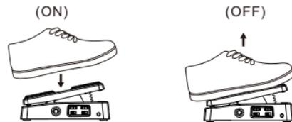
**SWITCH:** Place your foot on the pedestal and put it in "toe down" position. Apply slight downward pressure to activate the effect. Follow the same method to deactivate the effect.
